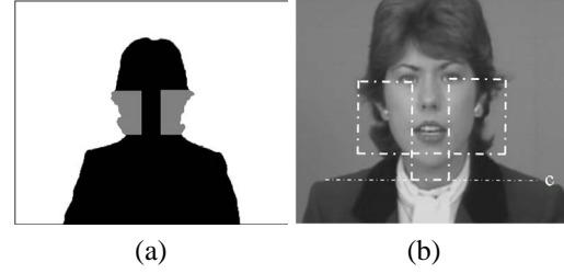
Fig. 5. (a) Segmented left cheek border region and segmented right cheek border region. (b) Rectangular search regions for the chin and cheek borders.
