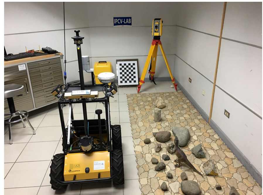
Clearpath Robotics Husky A200 rover platform and Trimble S3 robotic total station used for the experiments.
