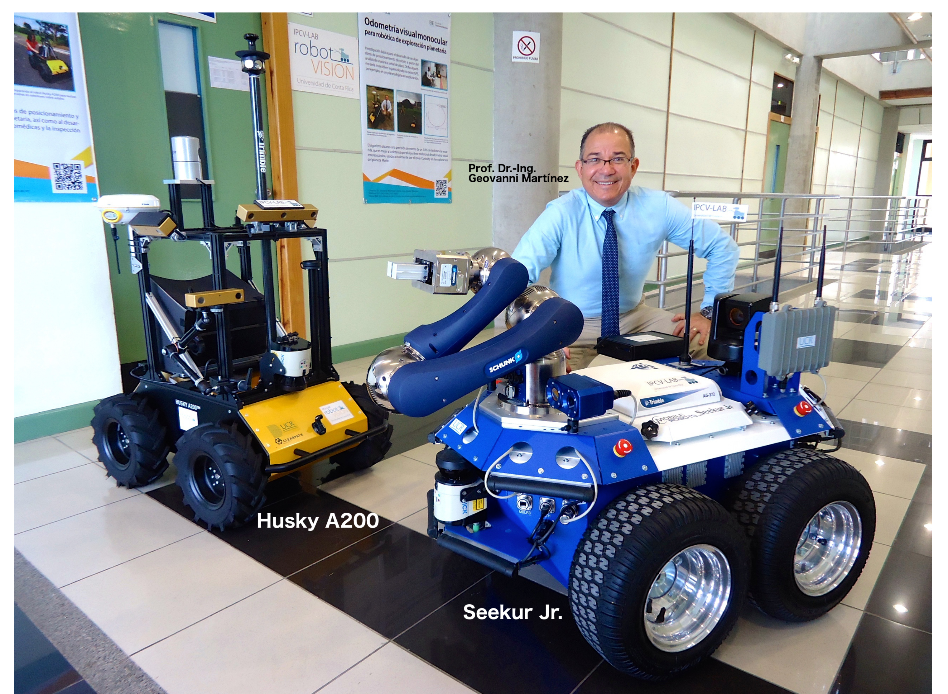
Figura 1: Robots used to test the new NIR ToF odometry and SLAM technologies developed at the IPCV-LAB for autonomous navigation systems.
